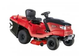
AL-KO PRO 450 Engine - 7.7kW / 452cc 95cm Cutting Width 310 Litre Grass Collector Hydrostatic (T3) Transmission Includes Mulch Kit, Bumper and Tow Hitch
