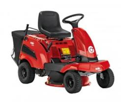
B&S 950E Engine - 4.0kW / 223cc 62cm Cutting Width 130 Litre Grass Collector Hydrostatic (T1) Transmission 25 - 75mm Central Cutting Height Adjustment
