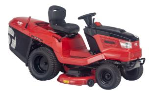
B&S Intek 8240 V-Twin Engine - 14.4kW / 724cc 125cm Cutting Width 310 Litre Grass Collector Hydrostatic (G700) Transmission Includes Mulch Kit, Bumper and Tow Hitch
